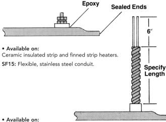
Mica insulated strip, ceramic insulated strip and finned strip heaters with leads.
