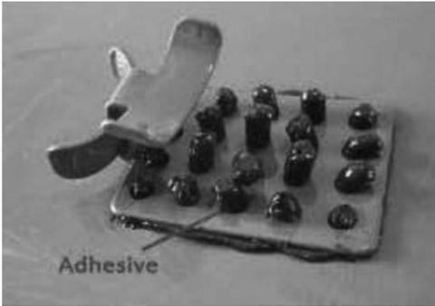
5. After the RTV adhesive has cured, install the heating cable between the clip clamps following the Cable Pattern Arrangement and Roof Clip Placement. Use pliers to close the clamps gently around the heating cable. **Do not crush the heating cable.**
