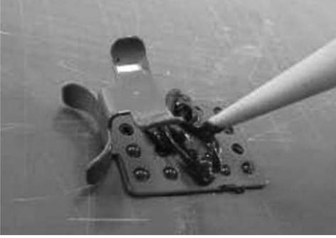
5. Allow the RTV adhesive to cure and dry before installing the cable. Refer to the RTV adhesive instructions for the cure time of the adhesive used.
