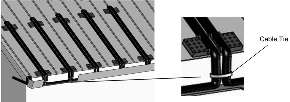
Clip Placement: Use 2 roof clips at the top corner points and 2 roof clips at the lower bottom corner points along the standing seam. Where the 2 ends of the cable meet at the base of each seam, they will be connected with a UV-resistant cable tie.
