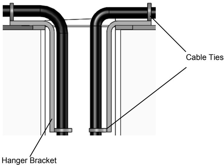
Two Hanger Brackets are used in each downspout to protect and provide stability to the heating cable. If you need more Hanger Brackets for additional downspouts, contact BriskHeat<sup>®</sup> for more information at 1-800-848-7673 (U.S. / Canada) or 1-614-294-3376 (worldwide).
