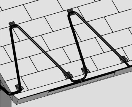
2. Following the RTV adhesive manufacturing instructions, apply RTV adhesive appropriate for your roof, to the back side of the roof clip where the nail or screw will be used.
