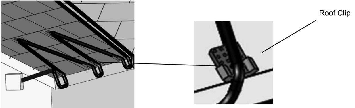
Clip Placement: Use 1 roof clip at each top corner point of the zig-zag and 2 clips at each bottom corner point.
