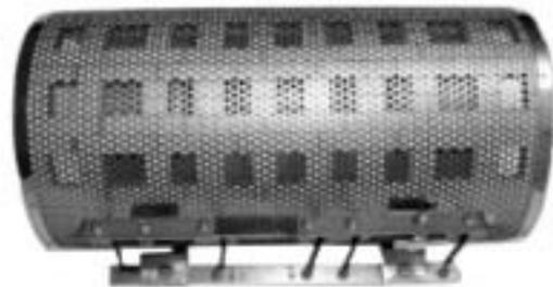
**MEGAFLEX** ceramic heaters can be combined with high velocity fans to form fast responding heat-cool units in accurate heating applications. These heaters are made with a perforated outside stainless steel sheath, and with no insulating jacket.
