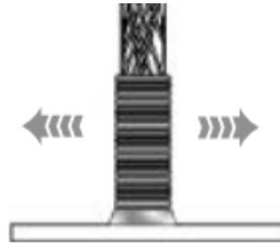
E Style SS braided leads with strain relief.
