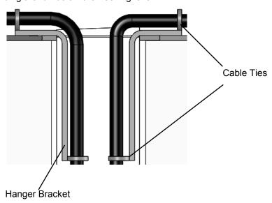
Two Hanger Brackets are used in each downspout to protect and provide stability to the heating cable. If you need more Hanger Brackets for additional downspouts, contact BriskHeat® for more information at 1-800-848-7673 (U.S. / Canada) or 1-614-294-3376 (worldwide).
