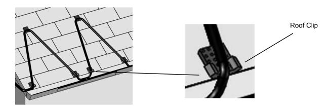
Clip Placement: Use 1 roof clip at each top corner point of the zig-zag and 2 clips at each bottom corner point.
