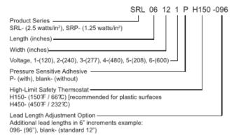
**IMPORTANT:** Temperature controller is required for this product. Contact OEM Heaters for options.
